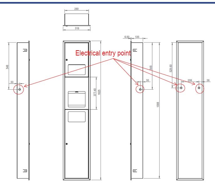
Please note: For installation of Metlam Australia Hand Dryers which have been hardwired by a qualified electrician, please ensure that an isolation switch is installed in accordance with current local codes or regulations.
